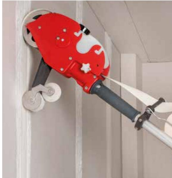
Once the compound has been applied, unroll the tape from bottom to top. Pull the trigger to cut the tape. You can now wipe down the tape.
